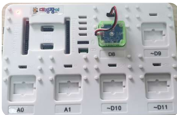
1.3.5-rasm. LED Blacksmith platadagi D8 piniga ulandi
